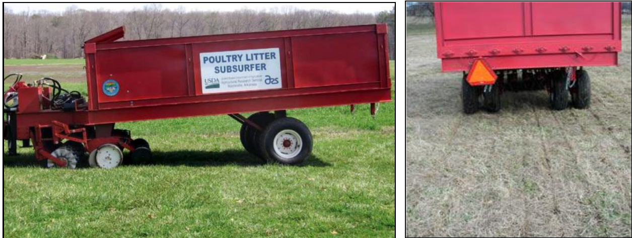
Figure 6. Left: USDA's Agricultural Research Service demonstrates a prototype poultry litter subsurfer in Arkansas. The subsurfer is designed to apply litter under the surface of perennial pasture and other no-till systems, and gives farmers precise control of litter application rates. Right: Subsurfer leaves a "clean" soil surface after application. Photos by Stephanie Jordan.
